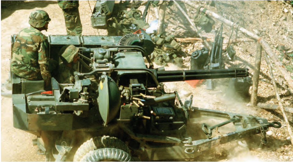
A U.S. soldier firing a Vulcan air defense system at a ground target
