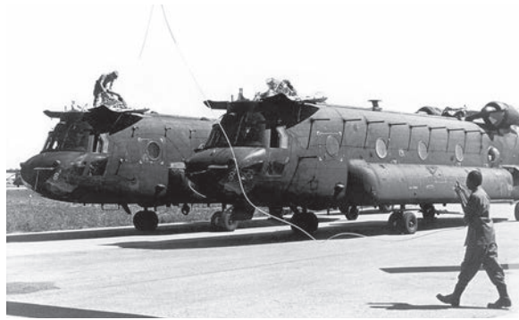
TOP LEFT: The rear pylon being removed from one of the two Chinooks. The maintenance crew had to ensure that each removed item, to include nuts and bolts, stayed with the airframe. TOP MIDDLE: The rear pylon after being removed from one of the MH-47Ds. The maintenance crew is placing it on a specially-constructed cradle that will accompany the helicopter onto the C-5A. TOP RIGHT: The two Chinooks have been disassembled prior to loading on a C-5A Galaxy. Both pylons and rotors had to be removed on each aircraft, to allow them to fit into the cargo bay. BOTTOM LEFT: The first of two Chinooks loading onto the C-5A for transport to Chad. The nose of the airplane pivots upward to allow access to the cargo bay. BOTTOM MIDDLE This photo demonstrates the tight fit for each MH-47D in the C-5A. The front and rear pylons had to be removed to provide enough clearance. BOTTOM RIGHT: One of the Chinooks is backed into the C-5A. A single Galaxy transported both helicopters and the 160th crew to Chad.
