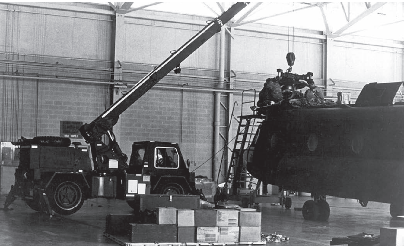
A Grove model RT41AA 4-ton Self Propelled Crane for Aircraft Maintenance and Positioning (SCAMP) is being used to remove a component from one of the Chinooks. A single SCAMP serviced both airframes.
