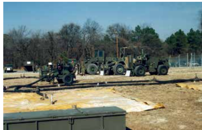
Fuel System Supply Point (FSSP) equipment, seen here on display at Fort Bragg, NC, had a considerably larger capacity than the more compact and transportable Forward Area Refueling Equipment (FARE). Both systems were used in Saudi Arabia.
