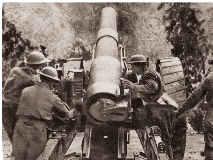
This 8-inch Mark 6 howitzer was used by U.S. Coast Artillery units in WWI and would have been familiar to SGT Munske. Because of its familiarity with heavy weapons, the Coast Artillery was tasked to provide artillerymen to the U.S. forces in France.
