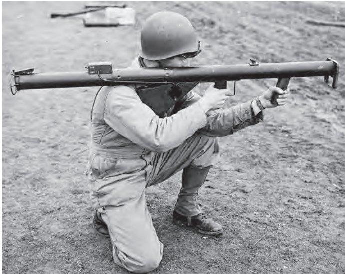
Soldier firing the M1 2.36" Rocket Launcher ('Bazooka'). The M1s weighed 18 pounds and were widely used against concrete bunkers in addition to light tanks/vehicles.
