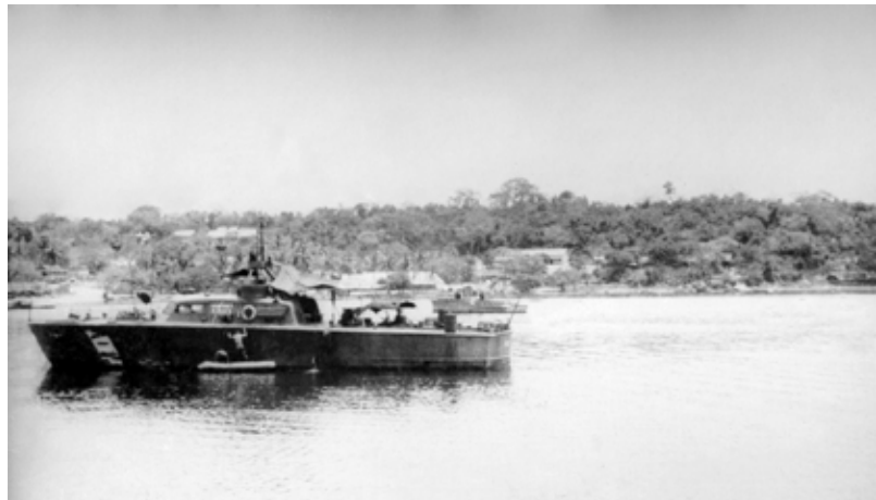
The three eighty-five-foot Air Rescue Boats formed the heart of the Maritime Unit fleet. Despite inadequate range and noisy operation, the boats were the principle craft for infiltrating agents and OSS personnel on the Arakan coast.
