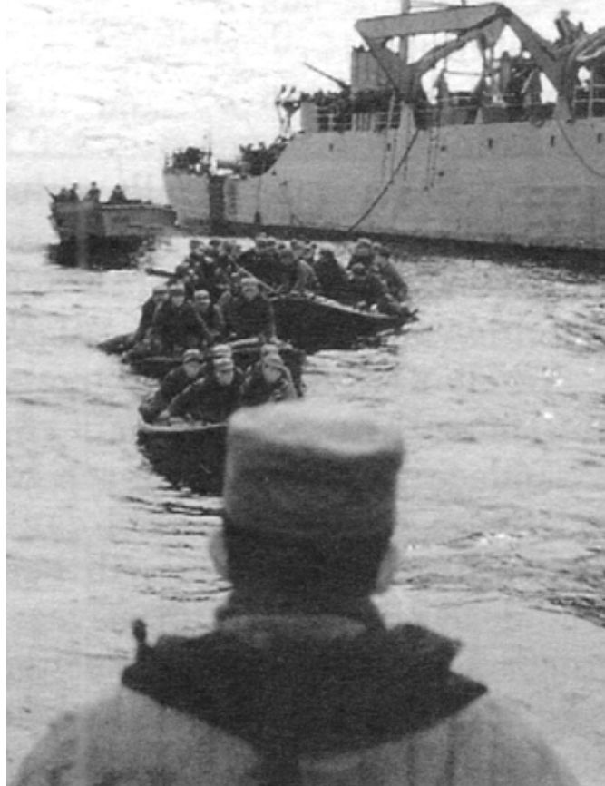
Marine Raiders and Underwater Demolition Teams had proved the utility of the four thirty-six-foot landing craft personnel, ramped (LCPR) carried aboard APDs (high-speed destroyer escorts) during WWII in the Pacific. The three APDs that supported JACK with LCPR were the Horace A. Bass (APD-124), Wantuck (APD-125) and Begor (APD-127).
