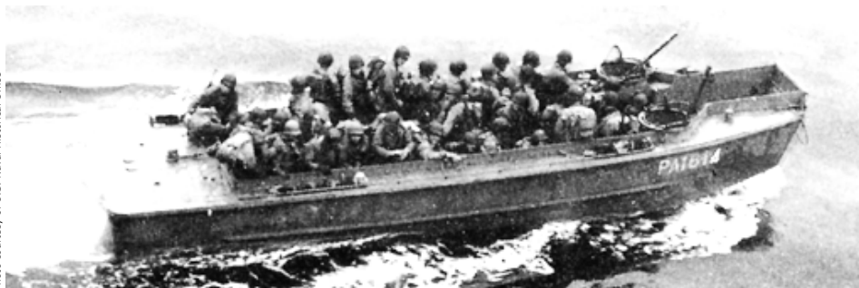
The 36-foot LCPR had two .30-caliber shielded machine guns on the sides of the bow, could reach nine knots fully-loaded, carried three crew, and thirty-six combat-loaded troops or 8,100 lbs. of cargo. The three and one-quarter-inch marine plywood hull afforded little protection, but its underwater exhaust system muffled the 225 hp Gray Diesel engine to facilitate covert infiltrations.
