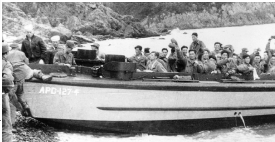
The 36-foot LCPR had two .30-caliber shielded machine guns on the sides of the bow, could reach nine knots fully-loaded, carried three crew, and thirty-six combat-loaded troops or 8,100 lbs. of cargo. The three and one-quarter-inch marine plywood hull afforded little protection, but its underwater exhaust system muffled the 225 hp Gray Diesel engine to facilitate covert infiltrations.
