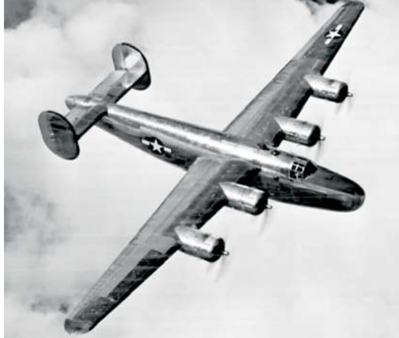
The C-87, as seen above, is the designation given to the cargo version of the B-24 bomber.
