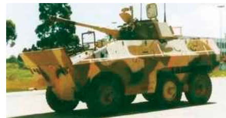
The EE-11 Urutu is a 6x6 armored personnel carrier that was designed by Engesa, a Brazilian company, in the 1970s. It can carry up to twelve personnel, in addition to the driver.
