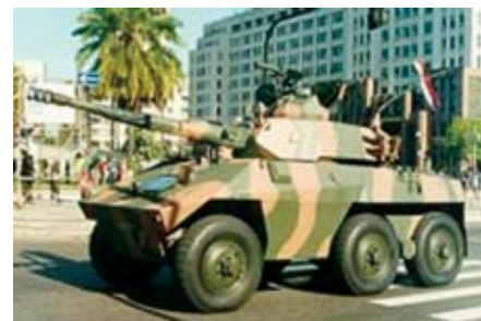
The EE-9 Cascavel armored car was developed by the Brazilian company, Engesa. It features a 90mm main gun, has a crew of three, and is extensively used by the Colombian cavalry elements.
