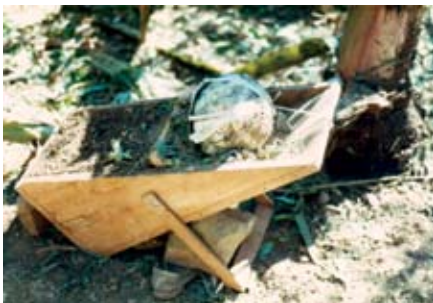
A close-up of artilleria sin cañon rampas showing wooden launchers with adjustable legs to set elevation. Earth was tamped against the backplate.
