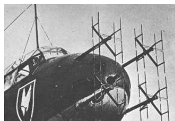
Top: German Junkers JU88G night bomber in flight; Left: Nose of the JU88G night bomber bristled with antennas; Right: German Messerschmitt Me110G4 night fighter with nose antennas.
