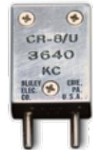
Actual size of a frequency crystal for Type A Mark III radio.
