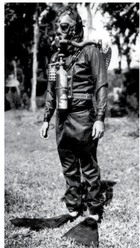
The Lambertsen Rebreathing Unit was the closed-circuit underwater breathing system used by the Maritime Unit.
