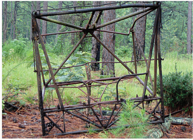
The photo on the left illustrates the pilot's compartment of the CG-4A Waco glider. On the right is the skeleton of another nose compartment which was pulled from a Camp Mackall swamp in the summer of 2006.
