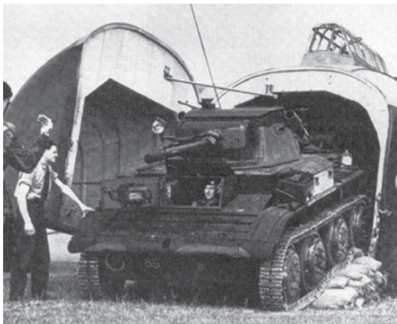
Tetrarch air delivered tank easing out of a British Hamilcar glider.
