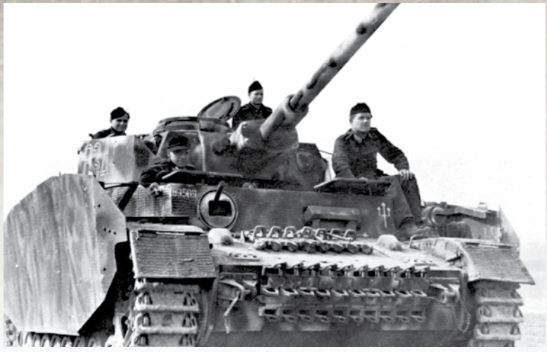
The Panzerkampfwagen IV had the added protection of armor sideskirts. Measures like these greatly increased the tanks' protection against anti-tank weapons.
