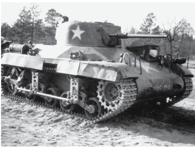
Front view of the M22 showing the 37mm main gun and .30 cal. machinegun in the turret. The driver's viewing port is raised.
