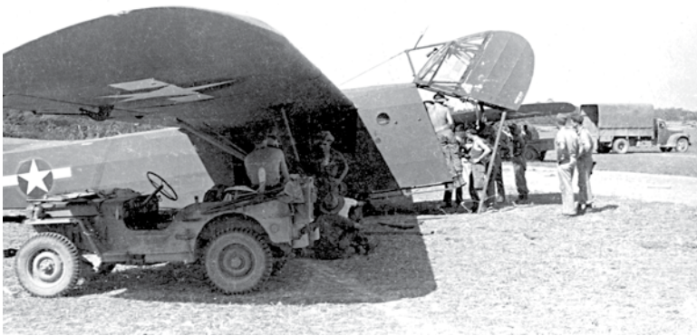
The CG-4A Waco glider was the basic U.S. Army glider of WWII. This example, being loaded by OSS Detachment 101 in Burma, has the nose flipped open to allow easier access.
