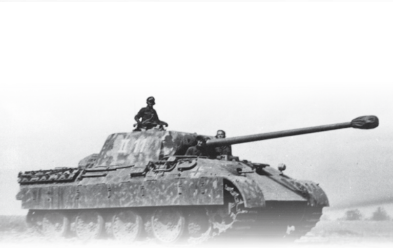
The Panther tank was intended to replace the Panzerkampfwagen IV. It was heavily armored, had sloped armor that decreased its vulnerability, and had a high-velocity 75mm main gun with tremendous penetrating power.
