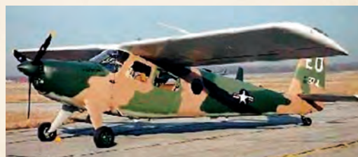
The L-28/U-10 "Super Courier," STOL (short takeoff and landing) capable, liaison aircraft was ideal for delivering propaganda leaflets and carrying civic action teams into remote areas of Latin America.
