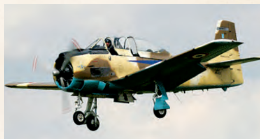
The T-28 "Trojan," a basic trainer for all U.S. services, was armed with machine-guns and could carry rockets and bombs for close air support (CAS) missions.
