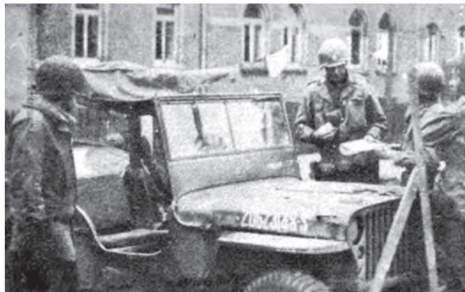
76th Infantry Division jeeps had a strong, four-foot V-shaped, angled bar welded to their front bumpers to foil German attempts to behead Americans with wire strung across the roads.
