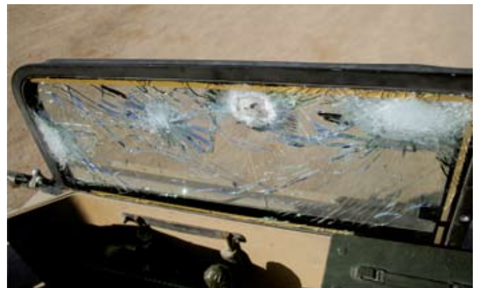
Proof of the effectiveness of ballistic glass mounted on the sides of the TF Raptor GMV cargo areas.
