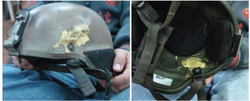
Outside & inside views of 7.62mm impacts on "MICH" helmets worn by ODA 563 soldiers. Both men survived with minor concussions.
