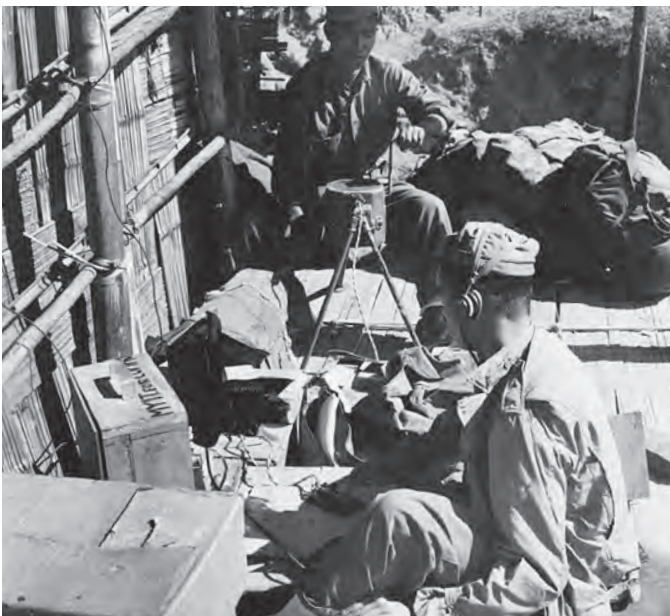
A Detachment 101-trained indigenous radio operator contacts headquarters in 1944, while another guerrilla turns a crank to supply power. Many of the radio operators had little to no English language skills but were very efficient in sending and receiving Morse Code messages.
