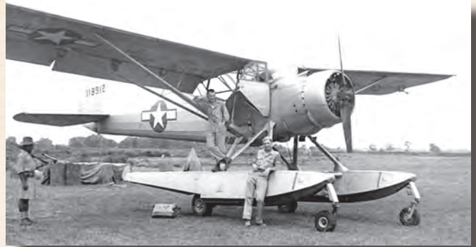
A Detachment 101 operated Stinson L-1 Vigilant. This one, nicknamed the "Burma Belle" has been fitted with floats to allow it to land on waterways.
