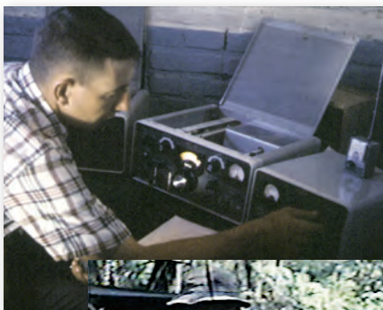
SFC Tom Carpenter, Heavy Weapons Sergeant, calls Panama on the Collins KWM2A commercial single sideband radio.
