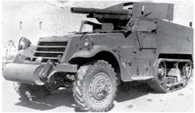
The M-3 half-track was intended to serve as a mobile anti-tank weapon (tank destroyer). The concept was abandoned after North Africa for larger vehicles with heavier guns. The Rangers used the vehicle for direct fire support.
