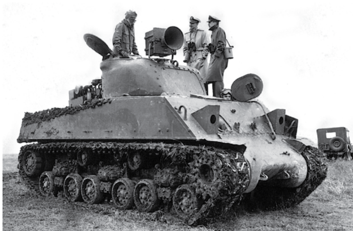
This M4A3 Sherman tank was modified for loudspeaker use.
