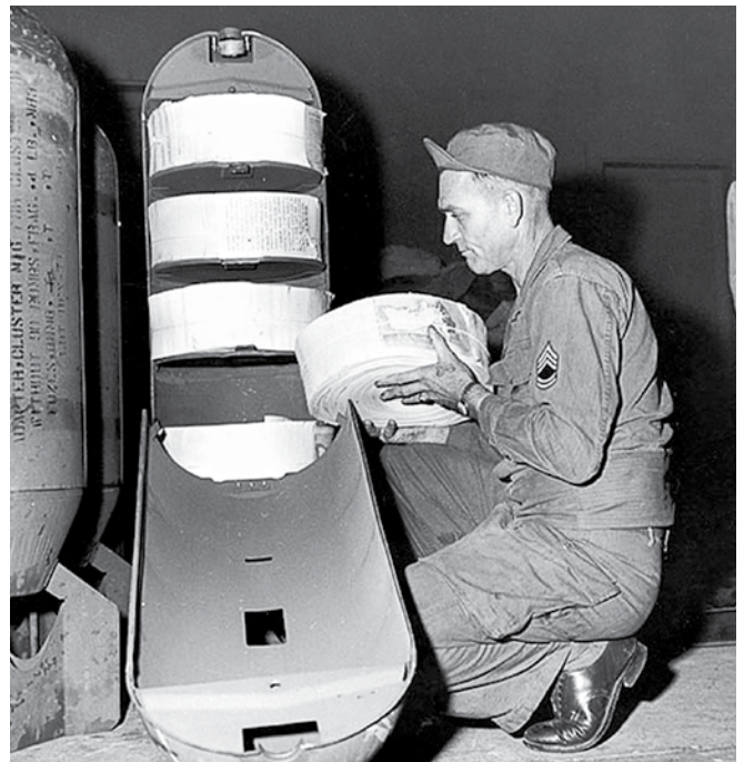
SFC Furl A. Krebs, 3rd Reproduction Company, loads an M16A1 cluster bomb adapter with 22,500 (5" X 8") rolled Psywar leaflets at the FECOM Print Plant. (U.S. Army, 1 Nov 1950)
