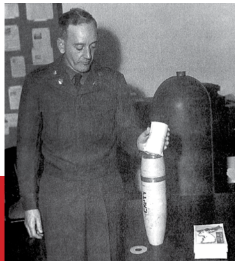
SSG Mason, X Corps Psywar, shows how a roll of 400 Psywar leaflets fits in a 105 mm howitzer smoke canister shell.
