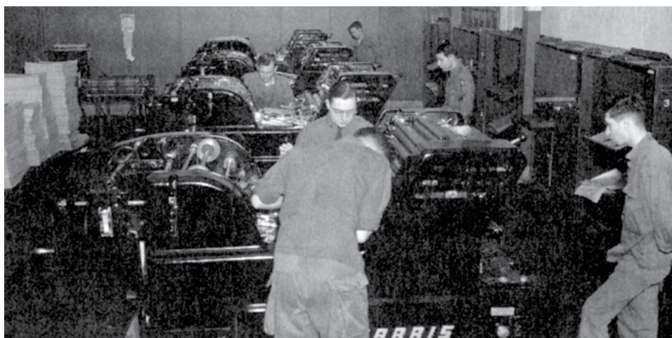
3 rd Repro Company pressmen working the Harris 17 x 22 inch presses at the FECOM print plant.
