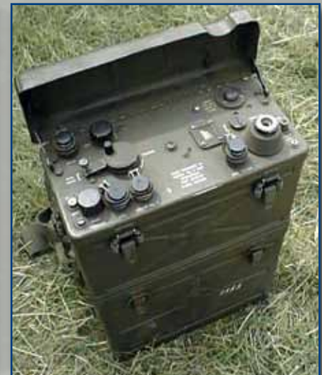
(Above) Short range (about 3 miles) SCR 300 FM radio was carried by the Korean guerrillas.
