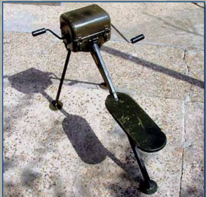
GN-58 hand-cranked generator for the AN/GRC-9.
