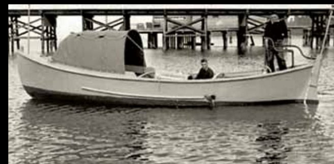
The 26 foot MKII Navy Whaleboat (NWB) was plywood. Its radar signature was almost non-existent, even when the canvas shelter was erected.
