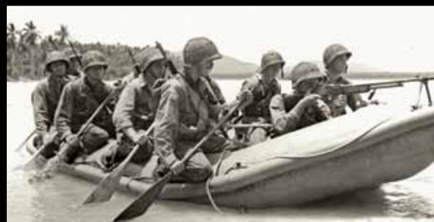
The LCRL or LCR (L) (Landing Craft Rubber Large) was an inflatable boat used by the USMC and US Army in WWII and Korea.
