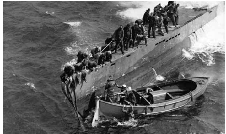
The carrying capacity of the Navy twenty-six foot plywood Mark II motorized whale boat (MWB) was limited. The coxswain normally stood to steer the craft. It is easy to understand why the coxswains were eager to break contact and get beyond small arms range.
