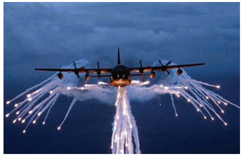
Figure 5.6 MC-130 launching chaff. The Combat Talons possessed a sophisticated system to avoid antiaircraft fires. Chaff and flares were fired from the aircraft to deceive incoming missiles.
