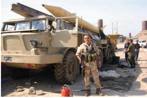
Figure 4.2 SCUD missile on launcher. Intermediate range missiles such as this were the prime targets of Task Force Dagger in the western desert. The threat of a strike against Israel drove the mission.
