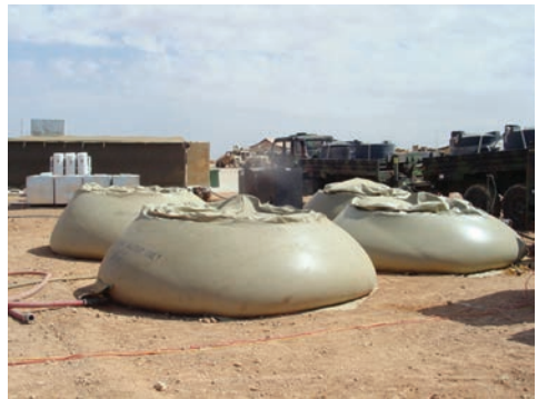
Figure 5.43 Fuel bladder at the FARP. Fuel bladders are a main component of the forward arming and refueling point operations.
