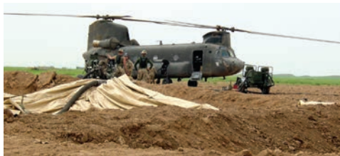
Figure 6.14 FSSP with onion skin. The BFSC, 528th Support Battalion, established fuel system supply points in northern Iraq in order to provide fuel support to aviation elements, such as the CH-47 helicopter shown here. Fuel pods, or "onion skins," are surrounded by earthen berms for protection and containment.
