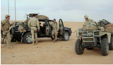
Figure 5.25 Modified NSV Tacoma pickup truck. The Toyota Tacoma was one of the most popular models of nonstandard vehicles in use by the Special Forces teams.
