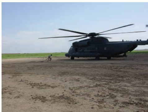
Figure 6.15 528th SOSB soldiers conduct a hot refuel of an MH-53.
