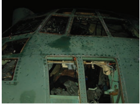
Figure 5.8 Windshield of MC-130. Antiaircraft fire shattered the windshield of the MC-130. Miraculously the crew landed the aircraft safely.
