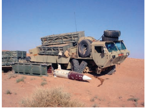
Figure 5.64 M977 HEMTT and loose HIMARS missile. During a night convoy, one of the HEMTTs hauling HIMARS missiles ran off the road. A missile broke out of the container causing some problems.
