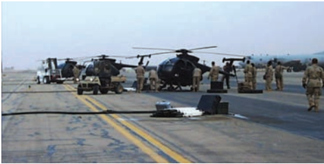
Figure 5.52 FARP operation. The rapid turnaround in refueling and rearming the Little Birds at the forward arming and refueling point was a key component of the success of the operations against the visobs.
