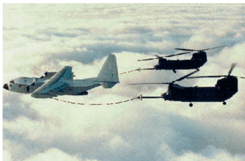
Figure 6.25 MH-47 aerial refueling from an MC-130P.
