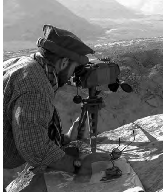
FIG 12. A Special Forces soldier employing a laser designator to mark targets for close air support.
