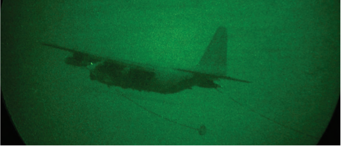
FIG 38. Night Stalker view of the C-130P trailing refuel lines and probe basket.
