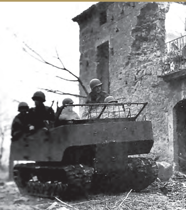
The FSSF Service Battalion maintained the M-29 Weasel, a tracked cargo vehicle designed specifically for the Force. An earlier T-24 model is pictured here near the Rapido River in Italy, 23 January 1944.
