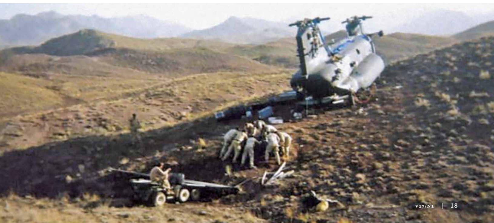
Bottom: Physically lifting the engines proved to be too much for the exhausted recovery crew, who had been working at high altitude for hours. They ingeniously used the Gator and the cut rotor blades to roll an engine into the back of the vehicle. Unfortunately, once on the Gator, they did not have the strength to lift it out, meaning that only one engine was recovered.
