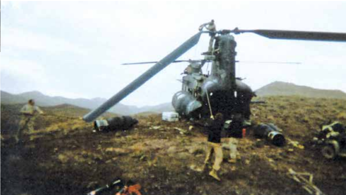
Left: The recovery crew at work cutting the rear rotor blades. Cutting them proved problematic and time-consuming when the blades bent down, forcing the crew to work them back and forth to help break them away.
