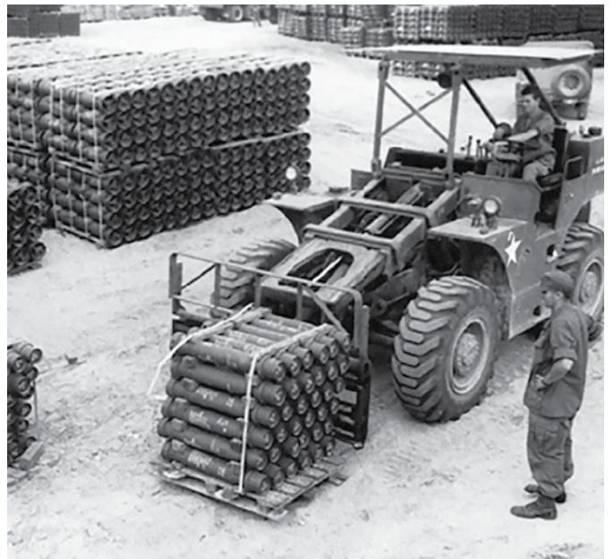
Top: Unidentified WWII Signalmen bury spiral-4 cable near the Rhine River. Bottom: 528th QMB personnel in RVN used 6,000-pound rough terrain forklifts to load, offload, and move ammunition and heavy ordnance.
