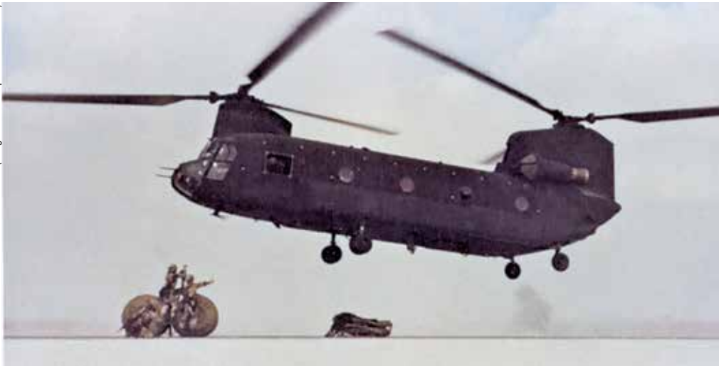
CH-47 helicopters delivered potable water, purified by 528th SOSB soldiers, to ARSOF outstations in Saudi Arabia using sling-loaded 500-gallon blivets.
